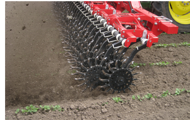
Rotary hoes can be operated at high speeds
